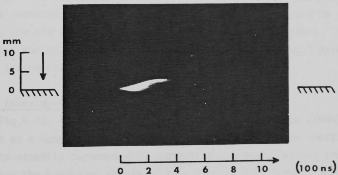
Fig.5.21. Streak photograph of plasma production from platinum in atmospheric air. Irradiance \sim 1.5 \times 10^8 \text{ W.cm}^{-2} . Camera aperture f/22 , 25dB neutral density filter.
