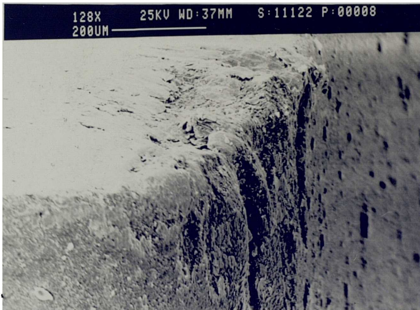
Fig 4.11 Wear grooves formed around the cutting edge of modified tool wear.
