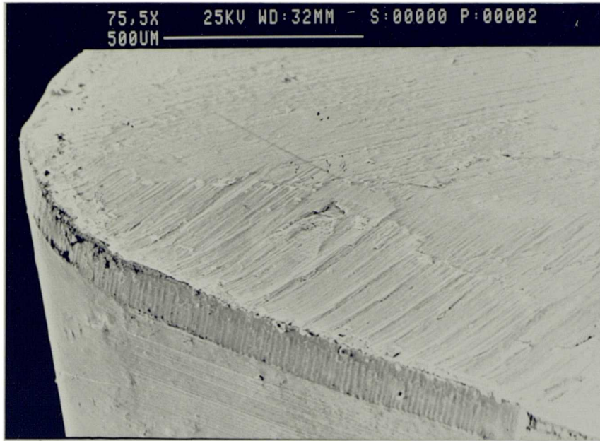
Fig 4.106 Worn surface of flank & rake faces of cubic boron nitride tool.
