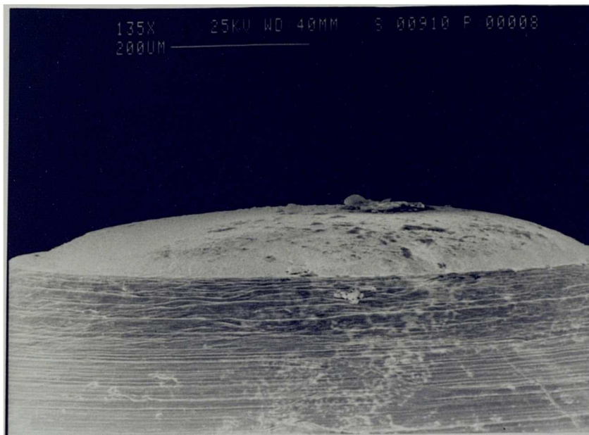
Fig 4.18 Titanium alloy indenter with strongly-adherent coated carbide (KC910) tool after fracture within bulk tool material.
