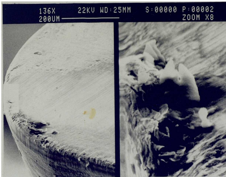
Fig 4.51 Smoothly worn crater surface by diffusion/dissolution wear.
