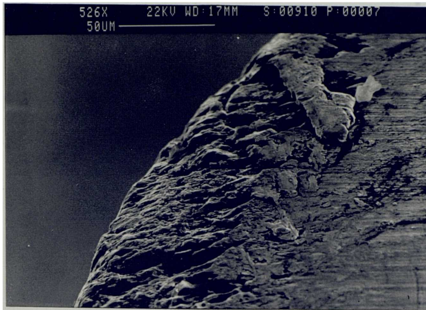
Fig 4.58 Plucking about to take place on the rake face of carbide coated tool.
