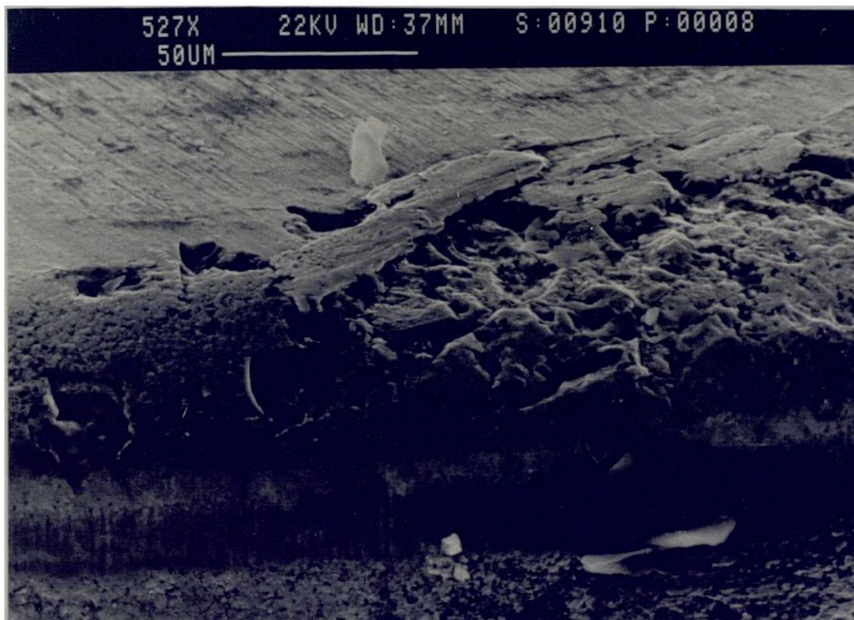
Fig 4.63 Smoothly worn flank face with plucking at the rake face.
