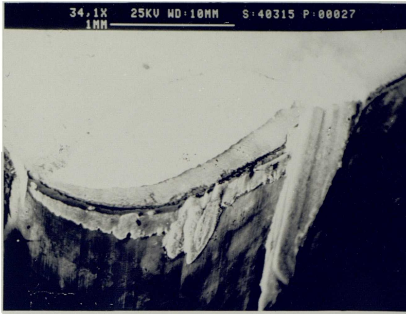
Fig 4.81 Development of notches at the both extremities of the depth of cut on the flank face.
