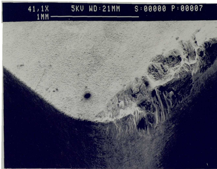
Fig 4.91 Chipping at the cutting edge of cubic boron nitride insert.
