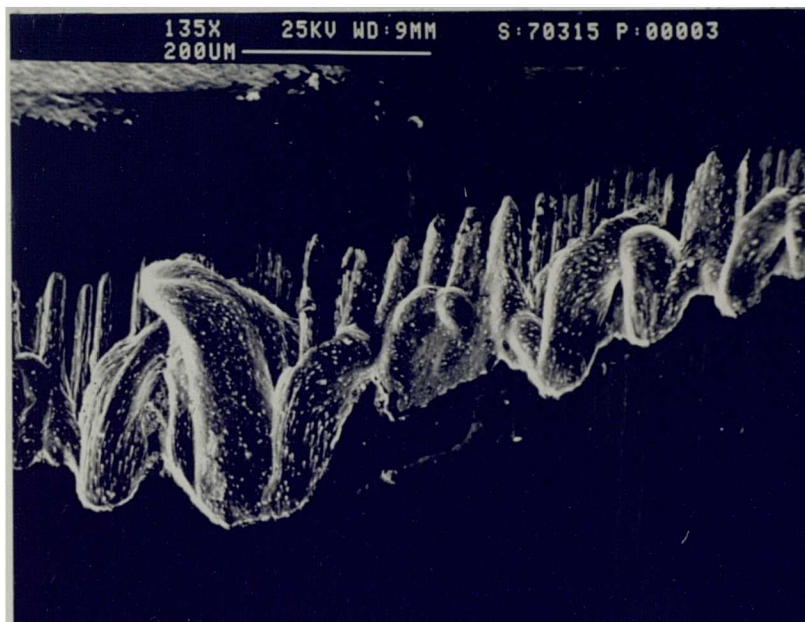
Fig 4.75 Showing WC particles detached from the cutting edge on to the flank face.
