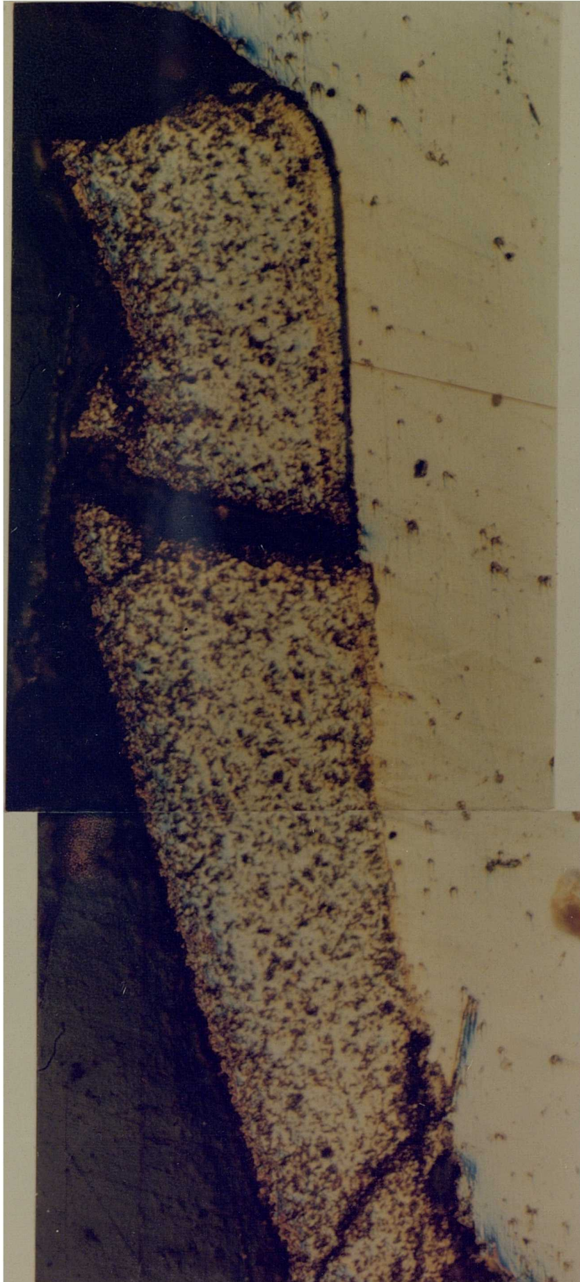
Fig 4.149 Section through 'quick stop' unetched specimen showing part of KC910 tool adhering to underside of chip(400X).
