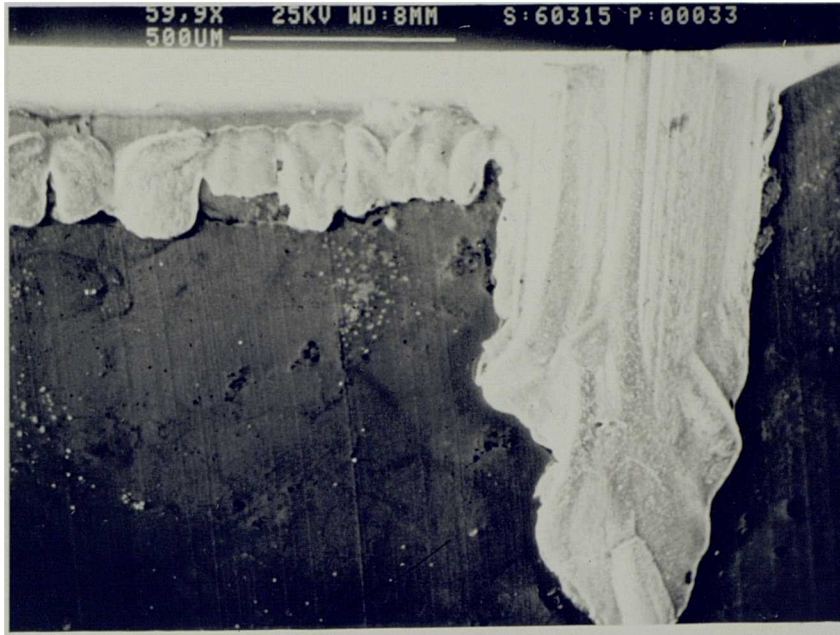
Fig 4.88b Formation of large size notch wear at the flank face.
