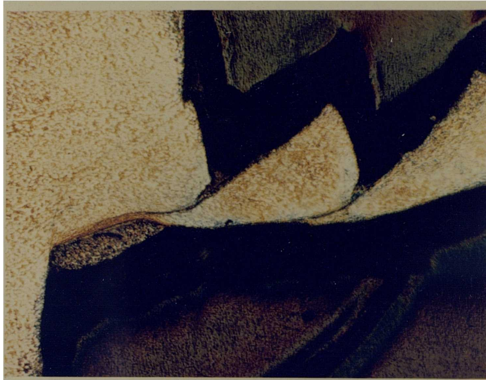
Fig 4.147a Section through 'quick stop' specimen showing part of cubic boron nitride tool adhering to underside of chip (100X).
