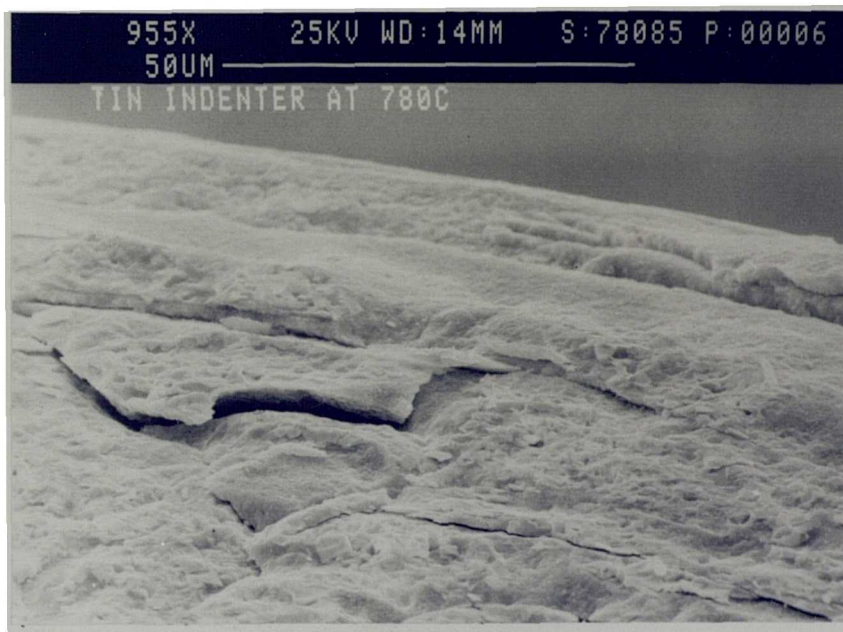
Fig 4.14 Titanium alloy indenter with strongly-adherent carbide (KC850) after fracture within bulk tool material.
