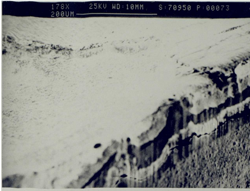
Fig 4.38 Wear on the rake face of coated carbide tool (KC850) as a result of attrition at speed of 75 m/min.
