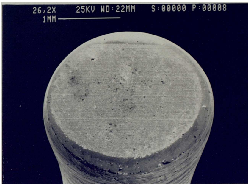
Fig 4.8 Titanium alloy indenter on the flank face of cubic boron nitride tool, showing no sign of adhesion.
