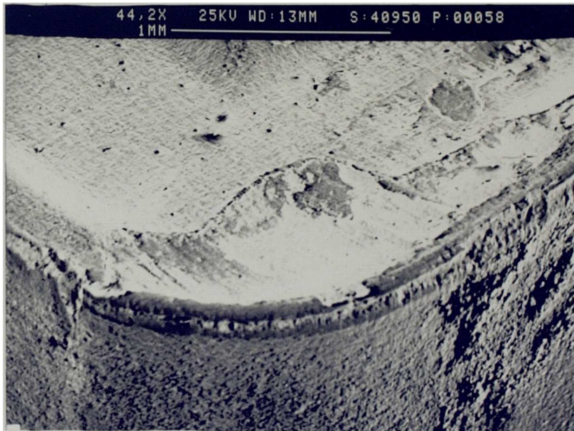
Fig 4.39 Formation of crater on the rake face of coated tool (KC850).
