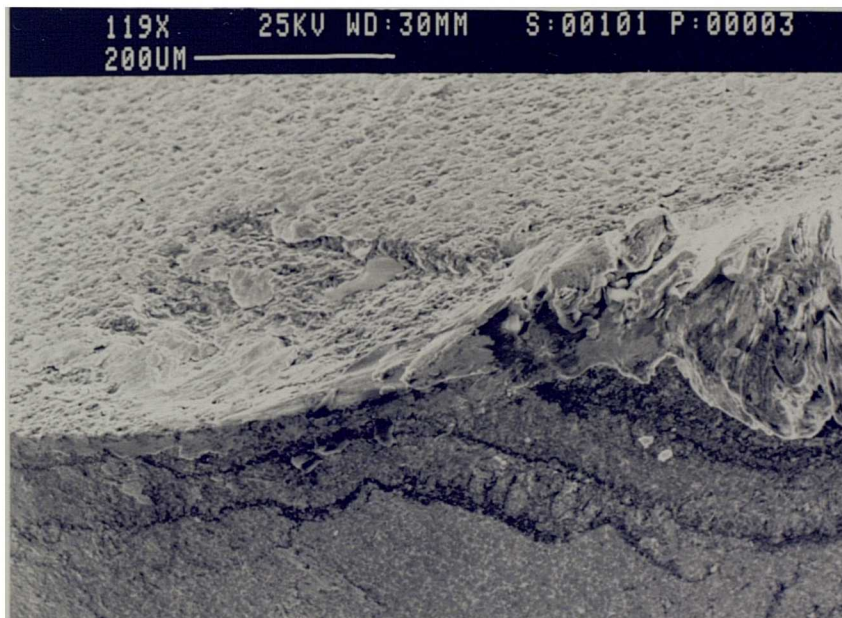
Fig 4.129 Formation of cracks on the flank face parallel to the cutting edge.
