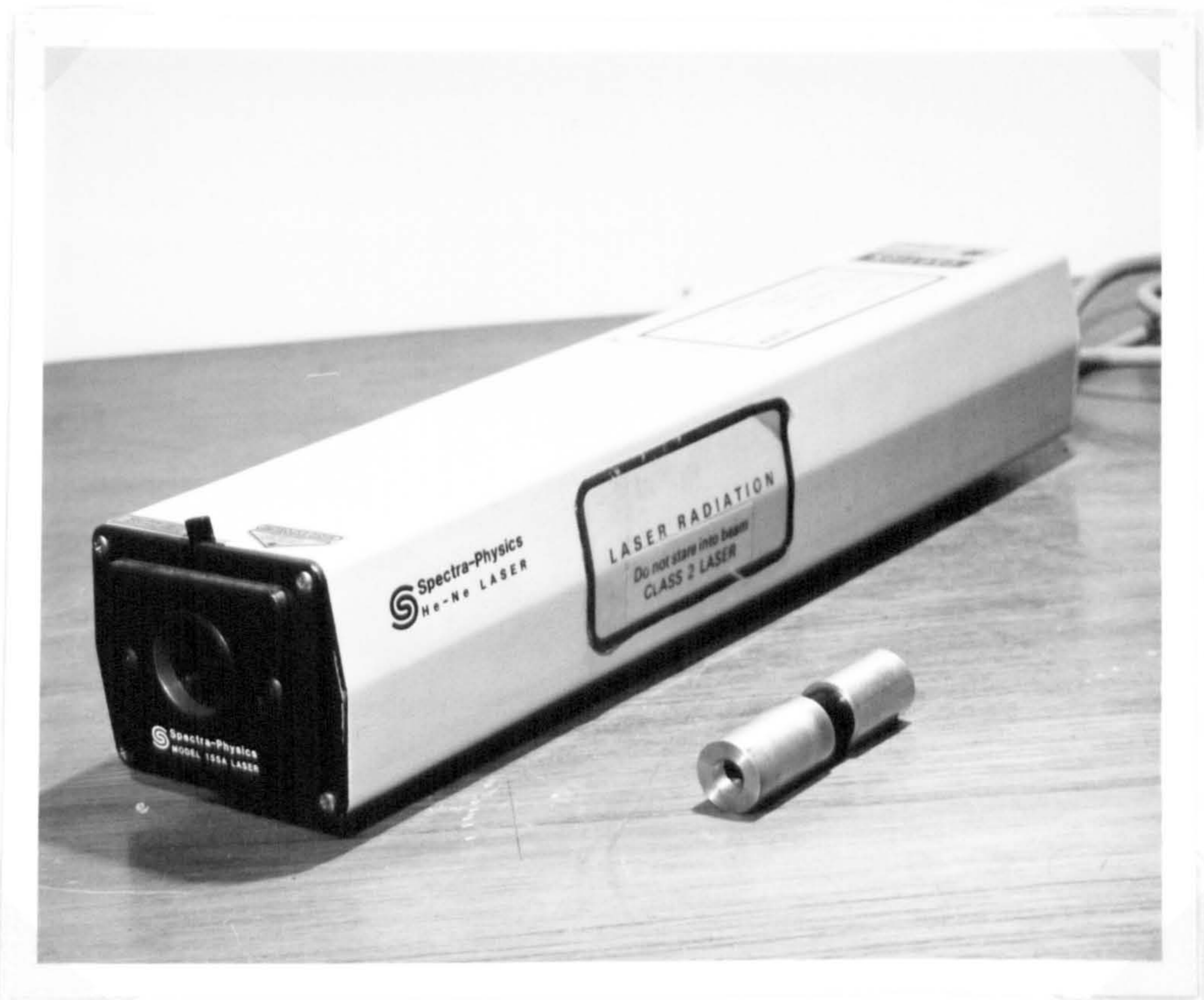
Figure 4-1 Comparison of a Diode laser (right) with conventional Helium-Neon laser (left)
