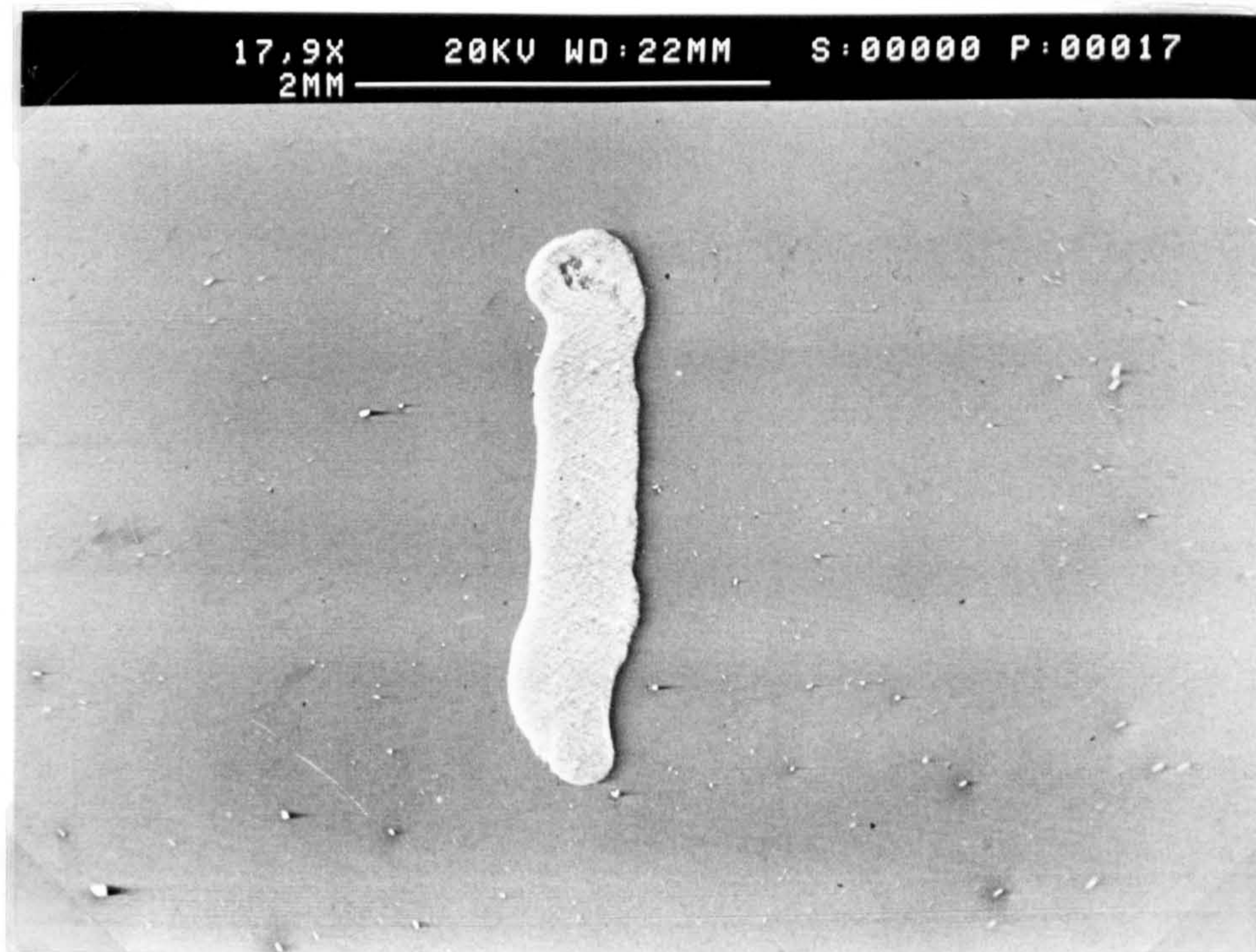
Figure 5-110 0.5 \mu\text{m} Polished sample with BUE defect, surface photograph
