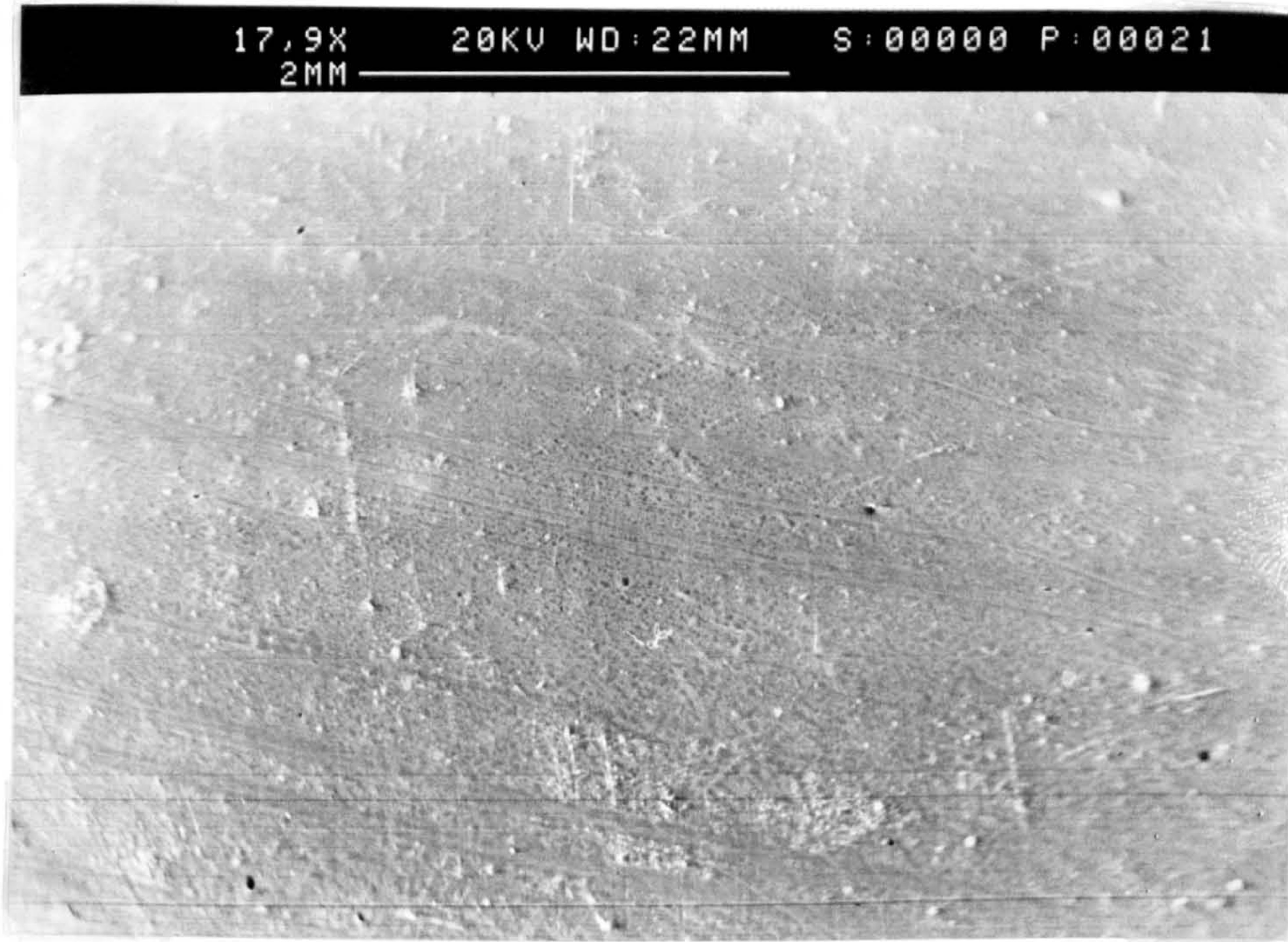
Figure 5-98 0.5 \mu\text{m} Plain polished sample, surface photograph
