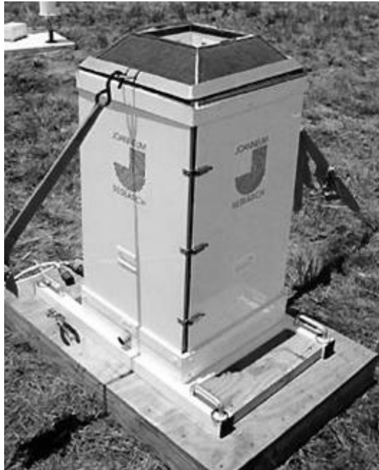
Figure 2.8: The 2D Video Disdrometer (courtesy of Kruger and Krajewski (2002))
