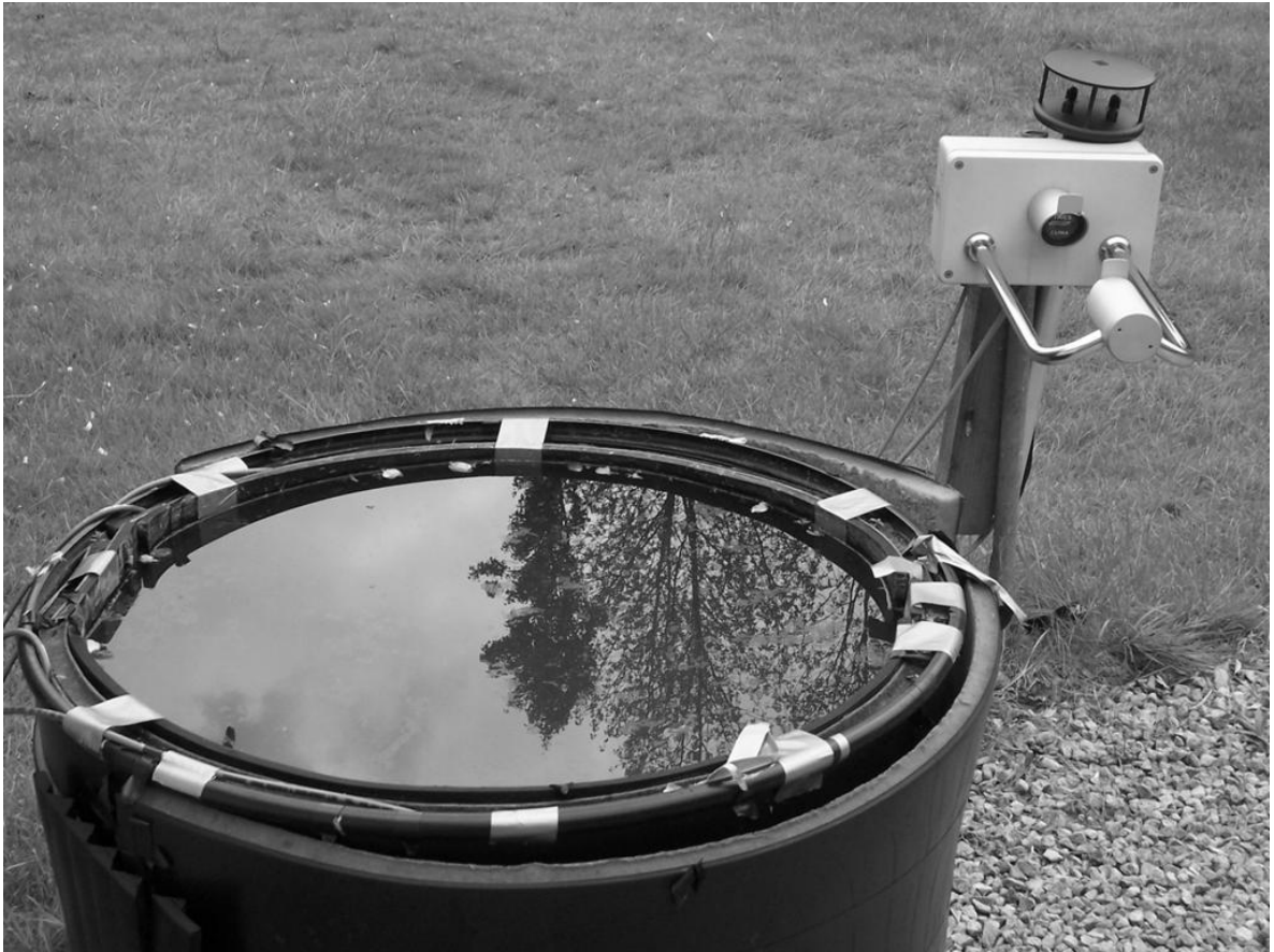
Figure 3.1: The experimental acoustic water tank disdrometer. PC and electronics located elsewhere for protection.
