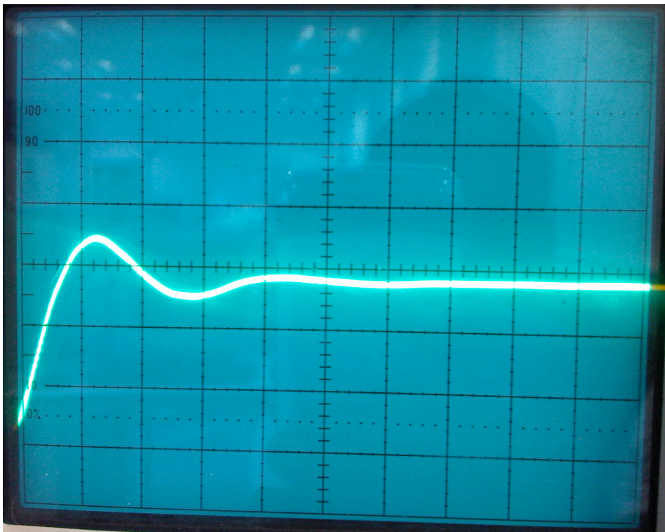
Figure 24: shows rise time of the received signal at 100kHz.
