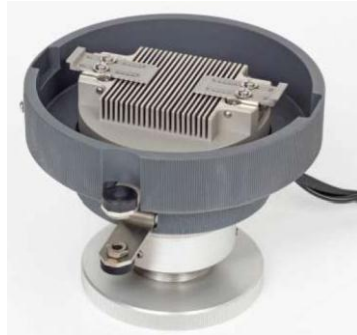
Figure 3.9: The work holder plate of the manual wire bonder.
