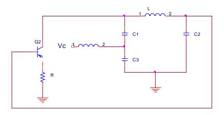
Fig 2.19: Resonant Oscillator (Best, 1997)
