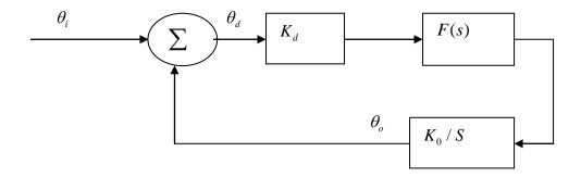
Fig: 2.6 Conceptual block diagram of linear PLL (Abramovitch, 1988)
