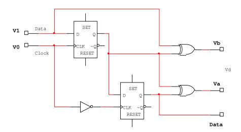
Fig 2.8: Linear clock phase detector (Best, 1997)
