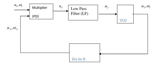
Fig: 2.2 Digital Phase-Locked Loop (Best, 1997)
