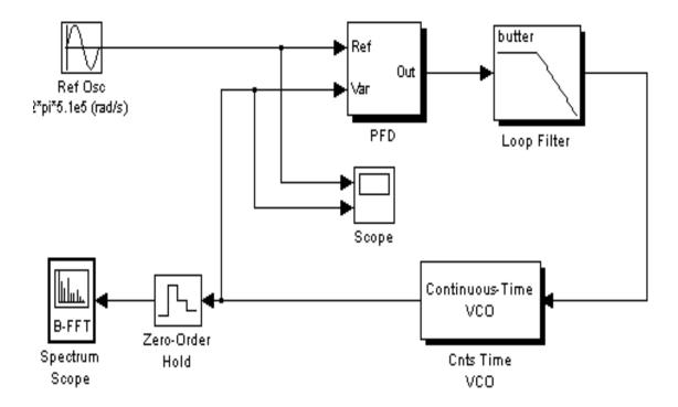
Fig: 3.1 Linear Phase-locked Loop
