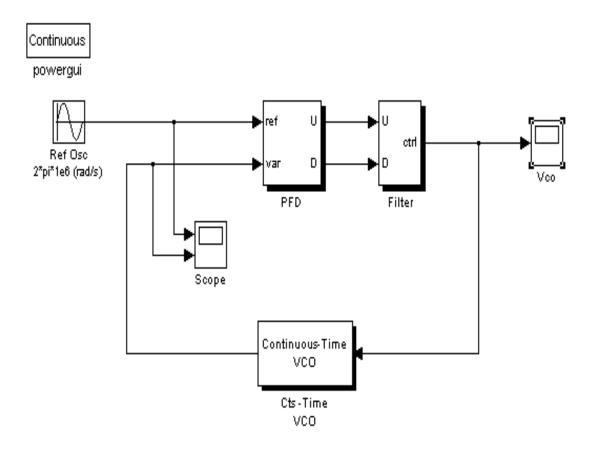
Fig: 4.1 PWR Phase-Locked Loop
