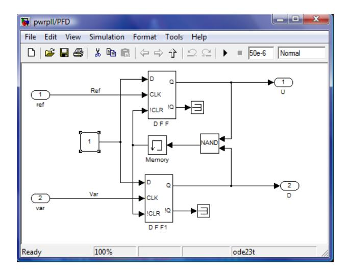
Fig: 4.3 Pwr PLL/Phase-Frequency Detector (PFD)
