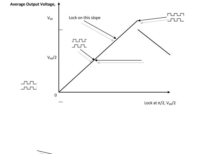
Fig 2.13: XOR phase detector characteristic at loop filter (Best, 1997)
