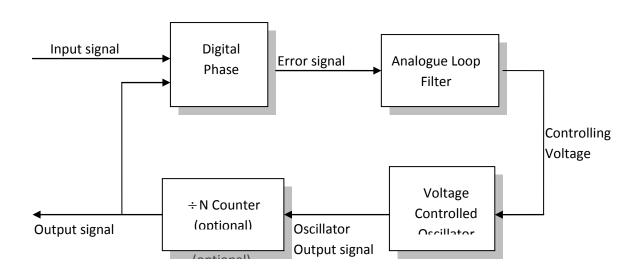
Figure 2.2(a): Fundamental blocks of classical digital phase-locked loop (Best, 1997)
