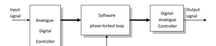
Fig 2.5: Conceptual block diagram of software phase-locked loop (Best, 1997)
