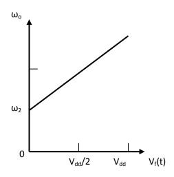
Fig 2.20: If  $\omega_{\mathrm{2}}$  required,  $V_{f}\left(t\right)=V_{dd}$  / 2 (Best, 1997)
