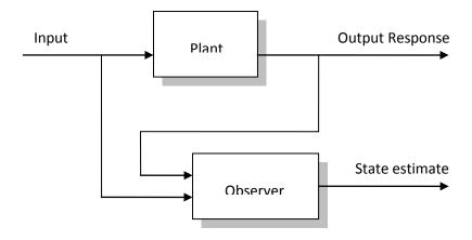
Fig 3.1: Feedback control system with observer attached (Roubal, 2006)
