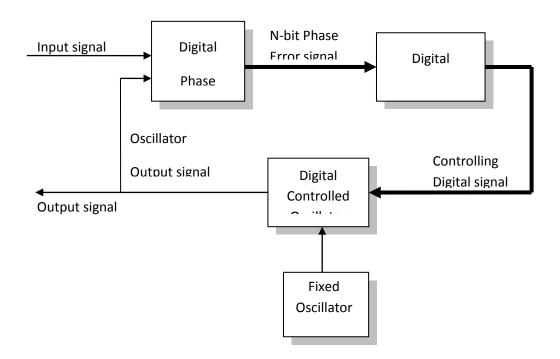
Fig 2.3: First version of all digital phase-locked loop (Best, 1997)
