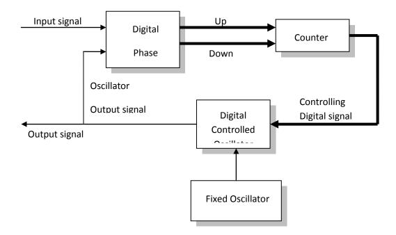
Mean while for the second version of ADPLL, as shown in Fig 2.4, it operates on a difference principle than the first version ADPLL, such that the digital phase detector generates pulses that go into count up or count down inputs of the counter which used to replaced the digital loop filter. The counter then enables and adjusts the frequency of the digital controlled oscillator.
