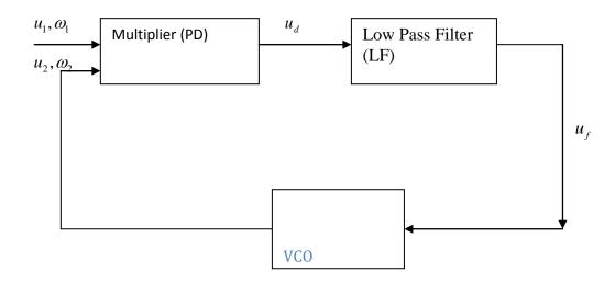
Fig: 2.1 Linear Phase-Locked Loop (Best, 1997)
