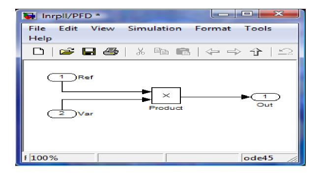
Fig: 3.2 Linear PLL/Phase-Frequency Detector (PFD)
