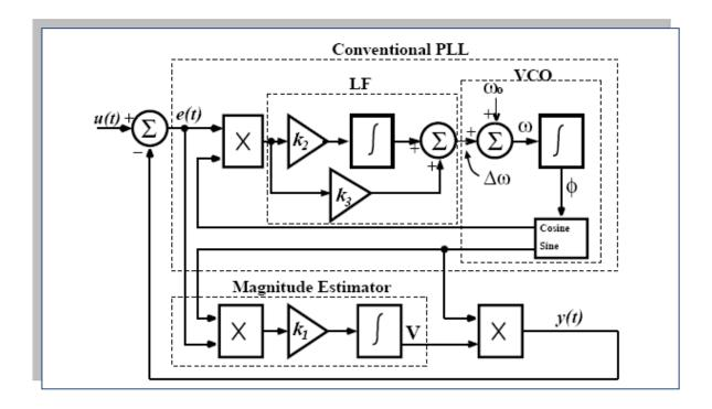
Fig 2.24: Conventional Phase locked loop (Lee, 1999)
