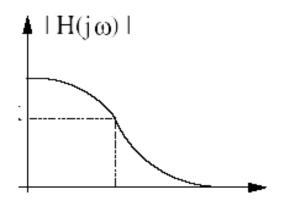
Fig 2.18: Cut-off frequency,  $\omega_c$  (or  $f_c$ ) (Best, 1997)
