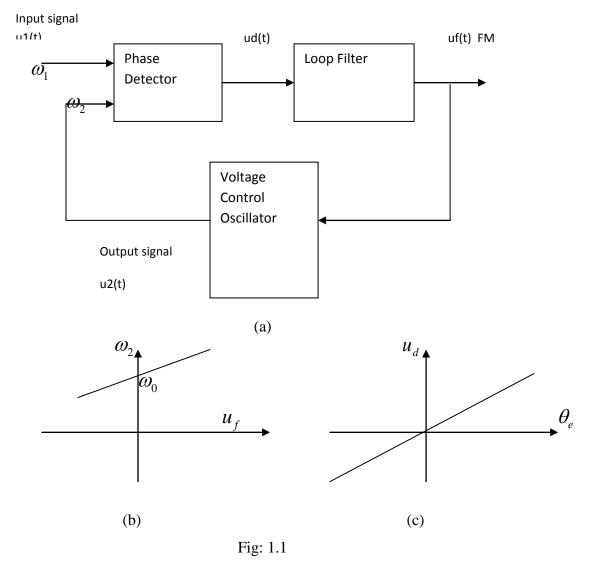
(a) Block Diagram of the PLL (b) Transfer Function of the VCO (  $u_f = \text{control}$  voltage,
