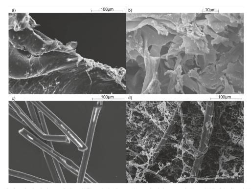
**Fig. 1 SEM images of microplastics before and after biofilm colonisation. a** Clean polyethylene terephthalate (PET), **b** biofilmed PET, **c** clean nylon, polyester and acrylic (NP&A) fibres and **d** biofilmed NP&A fibres. Note the scale in **b** is different than in **a**, **c**, **d** due to the higher magnification needed to visualise the biofilmed PET.
