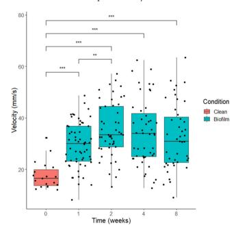
**Fig. 3 Changes in settling velocity of polyethylene terephthalate (PET) fragments over time (0–8 weeks) due to biofilm growth.** Clean particles are indicated by the red box while biofilmed particles are represented by the blue boxplots. The boxes represent the interquartile range where the line within each box represents the median and the whiskers represent the minimum and maximum. Brackets demonstrate statistical significance: \*\*\*p < 0.001 and \*\*p < 0.05 (n = 216).
