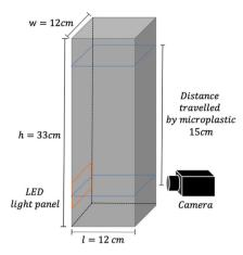
**Fig. 5 Schematic of the Laboratory Spectral Flocculation Characteristics (LabSFLOC) experimental set-up.** The set-up includes a plexiglass column of height 33 cm with a square cross section of 12 × 12 cm, filled with deionised water of varying salinities.
