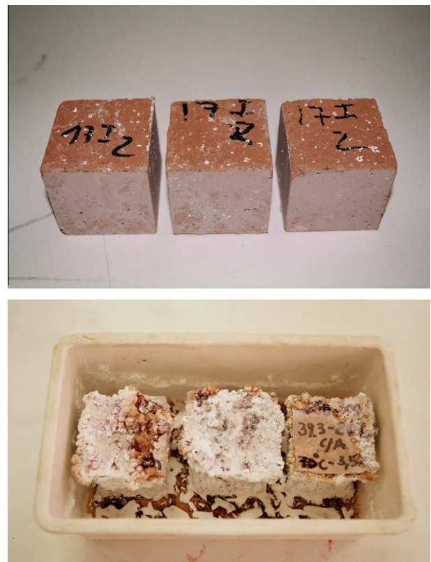
Fig. 3. Alkali-activated mine mortars specimens after water immersion: Above mortars based on plain mine waste mud calcined at 950 °C for 2 h; Below mortars based on mine waste mud calcined at different temperatures with sodium carbonate [67].
