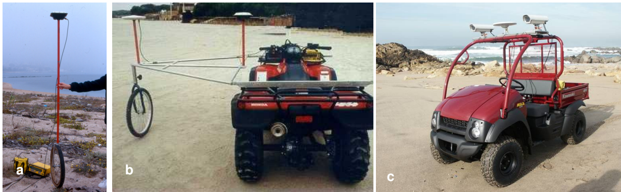
Fig. 3. Mobile mapping gear: a) single-antenna equipment; b) vehicle equipped with two antennas on an articulate arm, c) four-wheel vehicle with two antennas and videogrammetric equipment.
