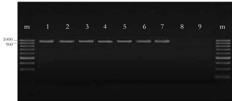
Figure 7. PCR amplification from P. brasiliensis 60855 using primers Hyg1 and Hyg2 (as described in Material and Methods). Lanes: m, 100 pb molecular marker; 1-6, P. brasiliensis transformants; 7, pUR5750 plasmid DNA; 8, P. brasiliensis wild type; 9, negative control. Positive reactions yielded a 982 bp fragment from hpb gene amplification.
