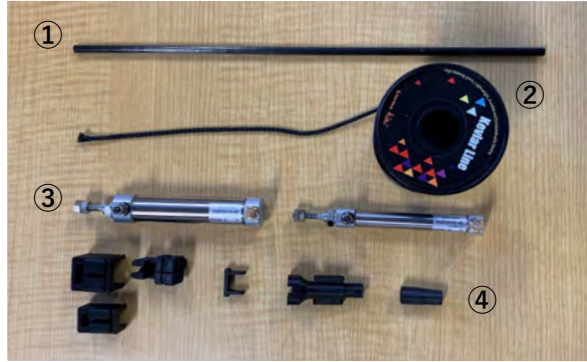
Fig. 3. Mechanical parts consisting of the developed tensegrity manipulator. No.1, No.2, No.3, and No.4 indicate strut, stiff cable, pneumatic cylinders, and connectors, respectively.
