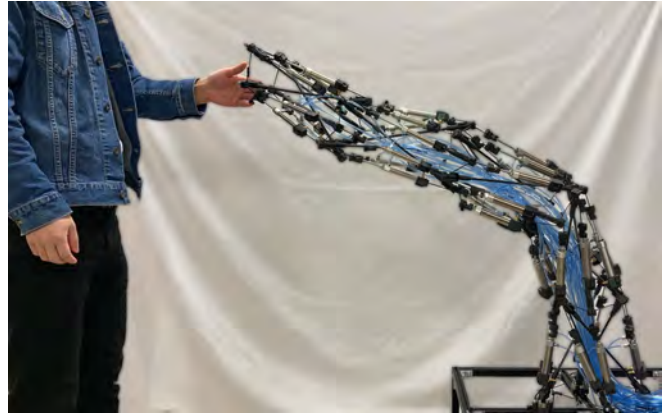
Fig. 1. The developed tensegrity manipulator. This robot is based on class 1 tensegrity and consists of 20 struts, 40 pneumatic cylinders, and 40 stiff cables. The height and mass are approximately 1.2 [m] and 3.5 [kg], respectively.
