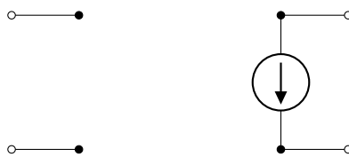
Fig. A.3 A small signal model of a FET.
