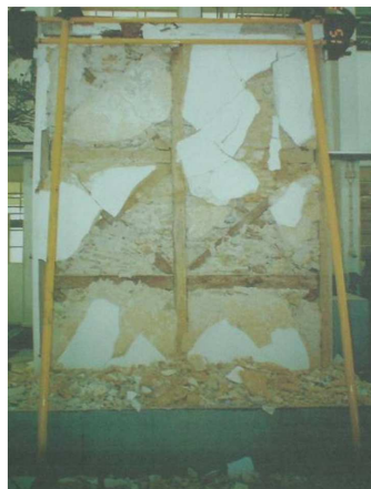
Figure 3 – Real wall specimen after test and hysteresis curves obtained (Langenbach 2007).
