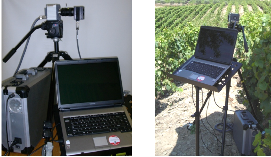
Figure 1. Spectral imaging system used to obtain the spectral data for the computations described in this paper.
