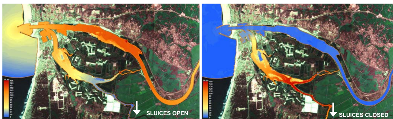
Fig. 18 Effect of Pranto River flow absence in RT values distribution (scenarios RT1 and RT6)
