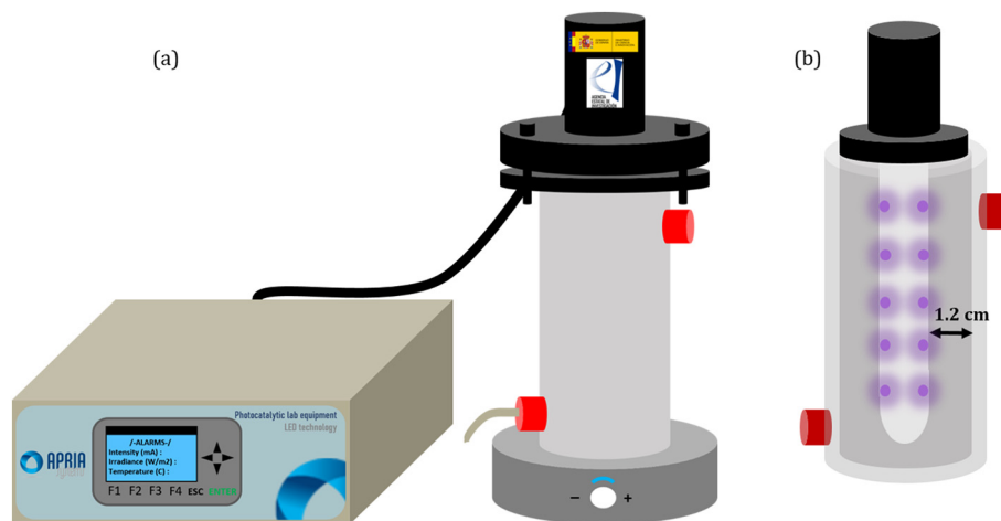
Fig. 1. (a) UV-C LED photo-reactor and control panel, (b) UV-C LED lamp inside the photo-reactor.
