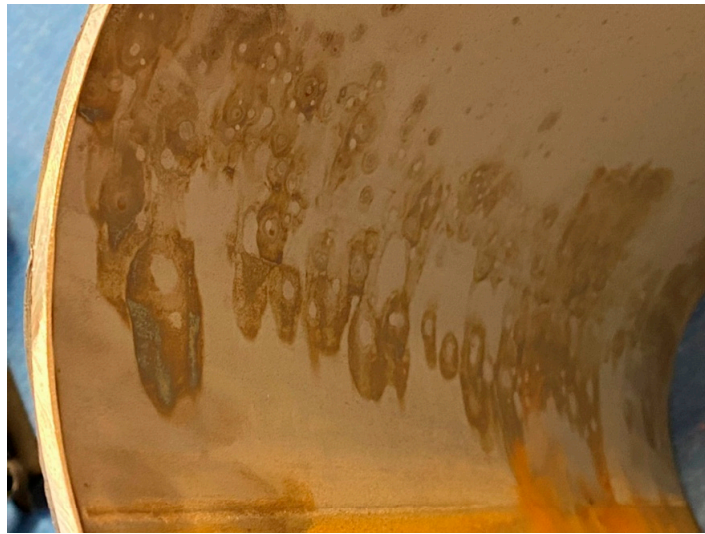
Figure 3. Multiple pitting onsets on the inside of the tube.
