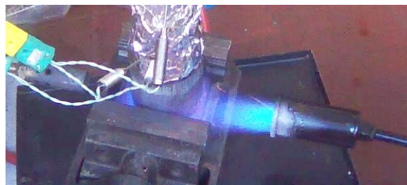
Figure 9 – Heating of the HP by 2 blow torches
