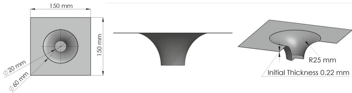
Fig. 2 CAD geometry and dimensions of experimental product
