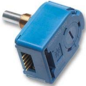
Fig. 9. Avago Technologies HEDS5700 encoder [11]
