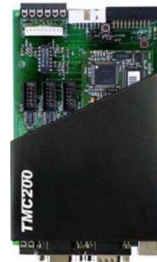
Fig. 4. TMC200 motion controller from Fraunhofer AIS
