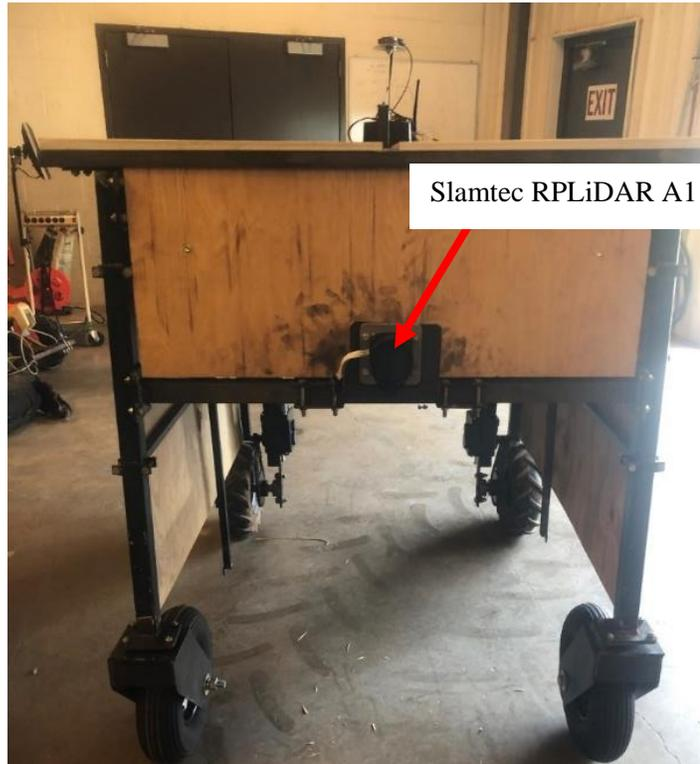
Figure 22 The rover with the LiDAR mounted on the front.
