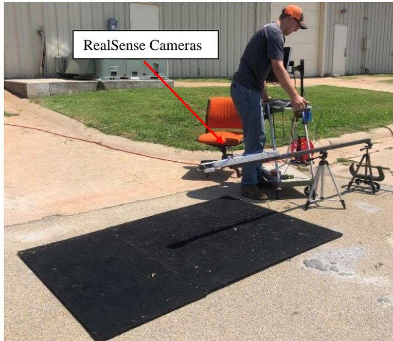
Figure 7 Test setup for the RealSense cameras
