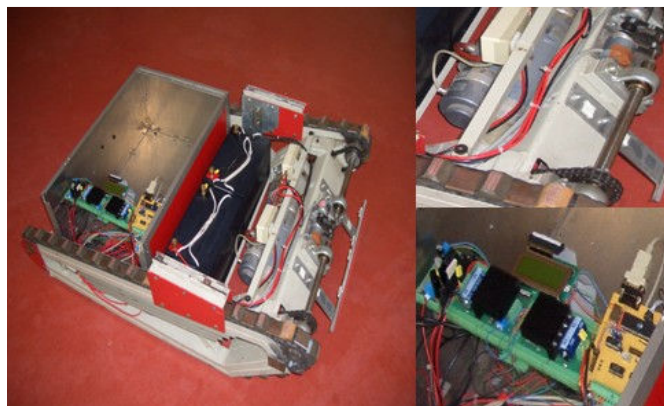
Fig. 1. Robot, DC converter, the microcontroller, display, batteries, motors, motor drivers and the encoders.
