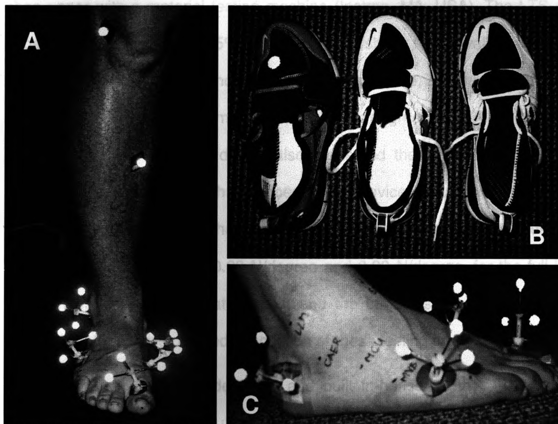
Figure 5.1. A) Location of the marker triad clusters on the foot. The base of the cluster remains affixed to the foot throughout the test protocol while the wand and marker portion is removed to allow for shoe changes. B) The three shoe types tested are the control (Nike Free trainer 7.0, left), the control shoe with a forefoot carbon plate attached to the midsole (middle), and the control shoe with a full length carbon plate attached to the midsole (right). All shoes have five holes cut in the upper at the heel counter on the lateral side, the toe box above the hallux, along the medial and lateral sides above the first and fifth metatarsals and on the medial side above the navicular tuberosity. C) Example of the anatomical landmarks that are digitized at the beginning of the test session. The landmarks form the anatomical co-ordinate systems for the dynamic trials. This is further explained in Jenkyn et al. 20
