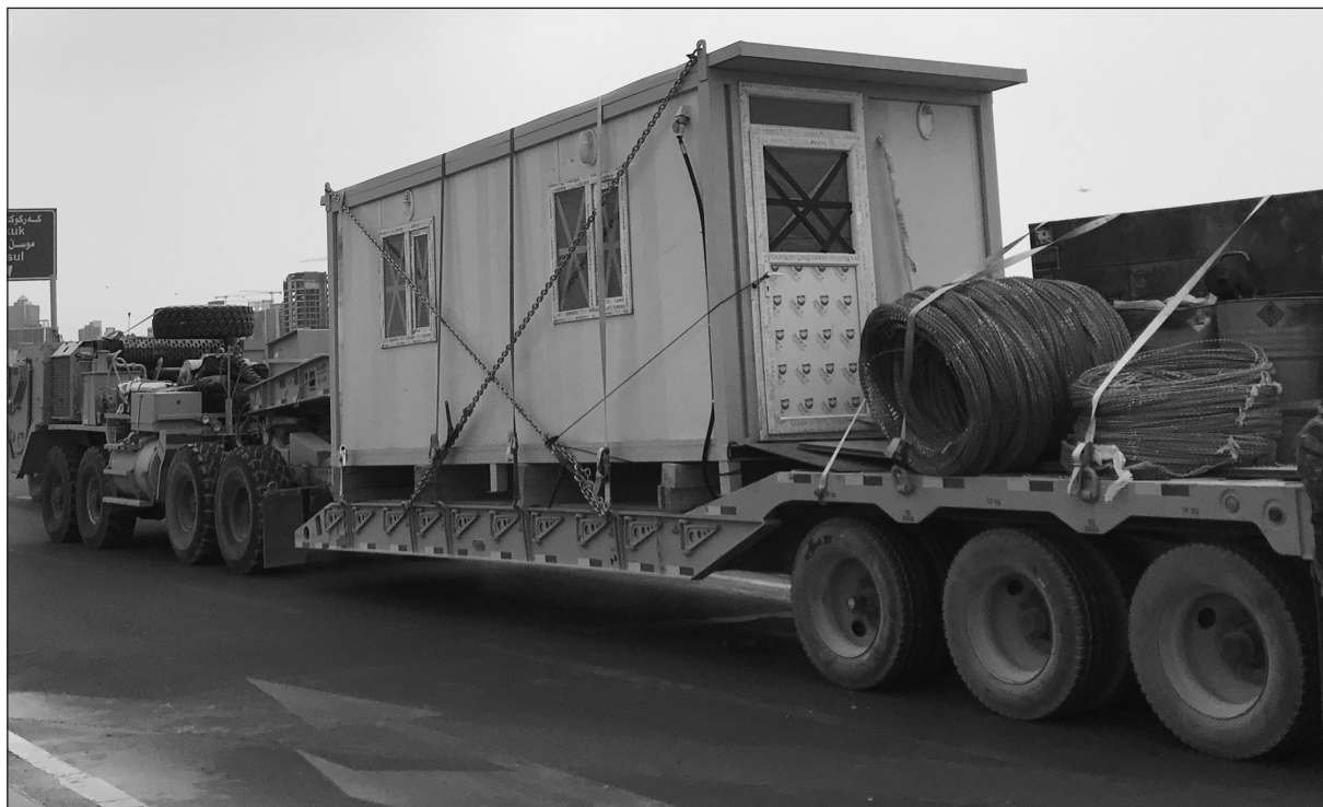
Fig. 1. Containerized housing unit (operating room) and generator fixed to an armoured tractor trailer.
