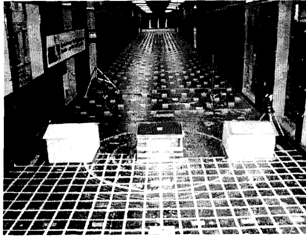
Fig. 3.1: Photograph of the 1:20 scale, gable roof model house in the wind tunnel, looking upstream. The house in the center is the main house.
