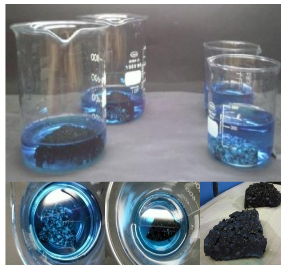
Fig. 4 - Images showing the samples immersed in the MB aqueous solution and sample's final aesthetics.
