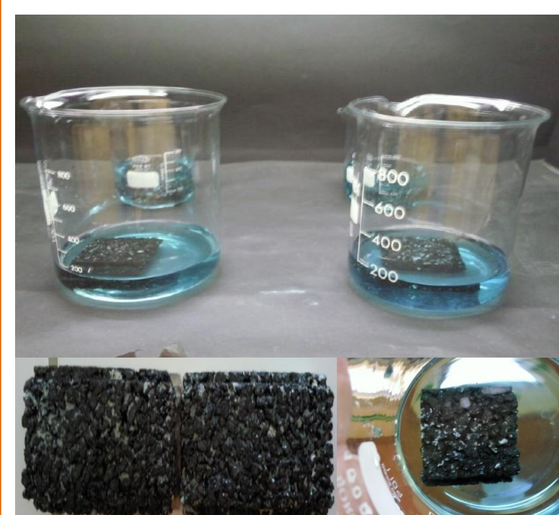
Fig. 6 - Images showing the samples immersed in the MB aqueous solution and sample's final aesthetics.
