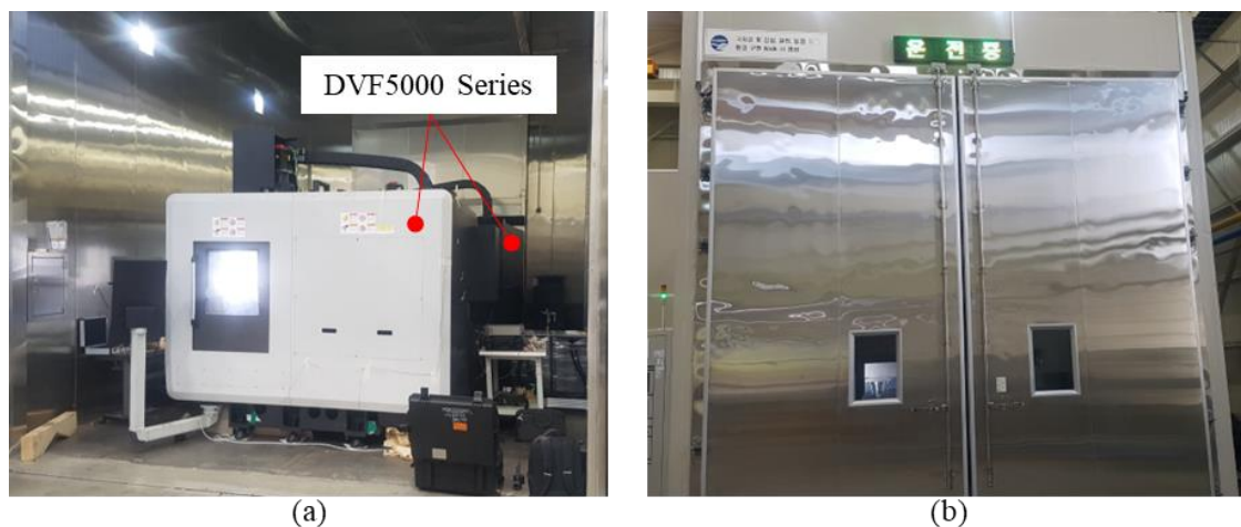
Fig. 5-1 Preparation for experiments using the environmental chamber; (a) installation of DVF5000 before tests, (d) state of the environmental chamber during the experiment
