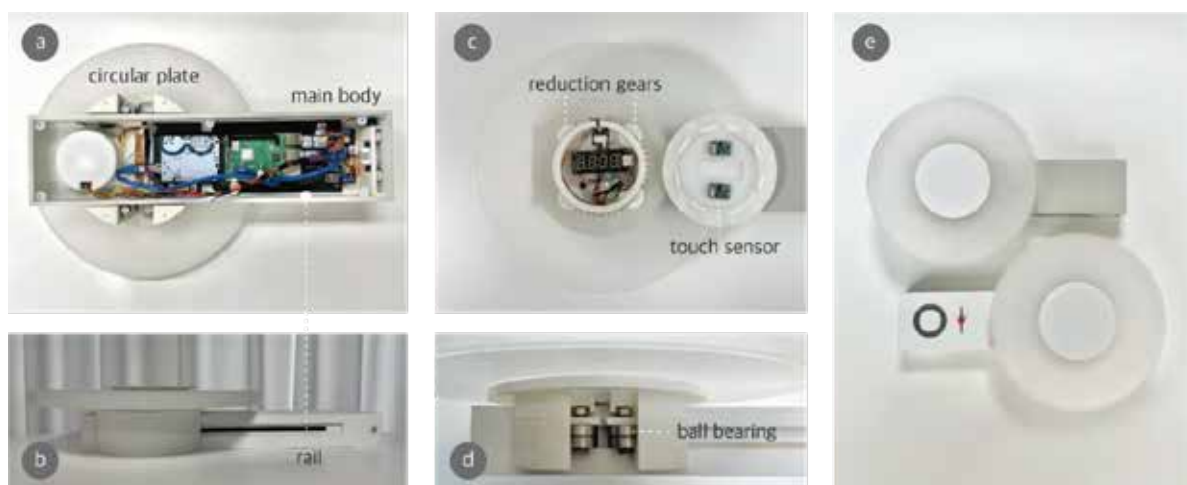
Figure 12. Detailed structure of Lumino: a) Lumino’s two main parts. b) The rail with a gap allows wires to move together. c) Circular plate structure. d) Ball bearings moving on a rail. e) Two Luminos with different colors.
