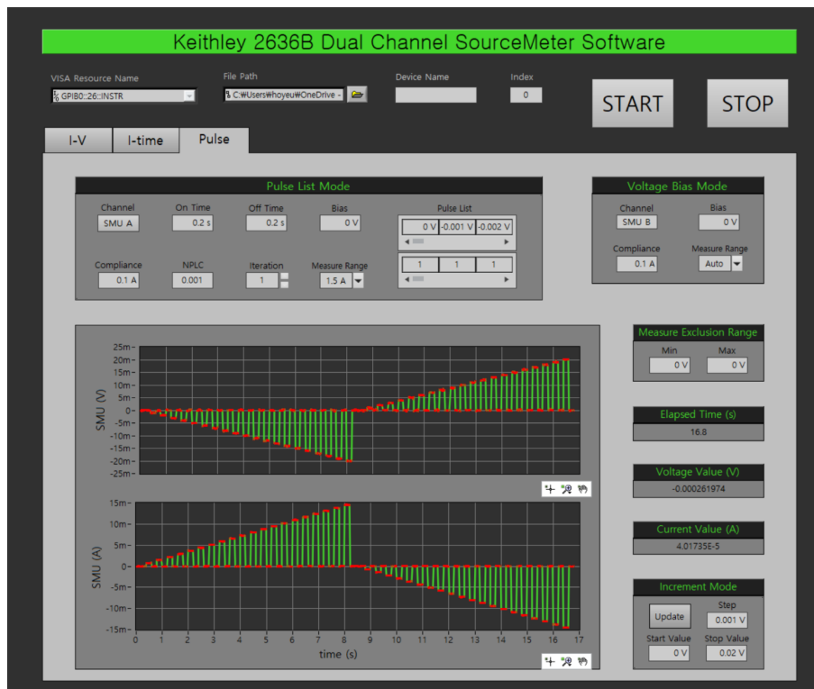
Figure 5.8. Keithley 2636B customized software using LabVIEW for synaptic measurements by pulse modulation.
