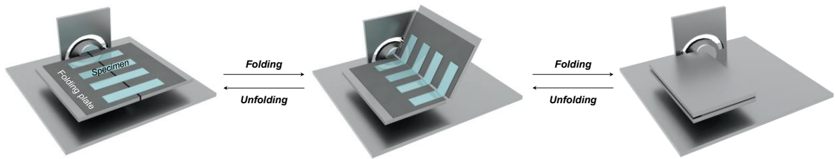
a) ■ Dynamic folding test of UV-blocking OCA
