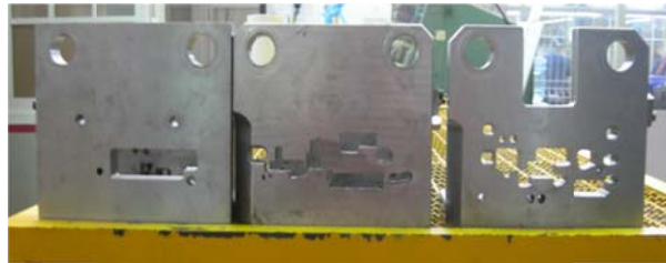
Figure 5: Non-standard support plates for dies
