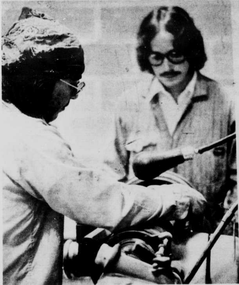
Students Larry LeCrone and Craig Anderson finishing honing a wheel cylinder by cleaning it with a brake fluid-soaked rag. William Annin, in white lab coat, checks the
