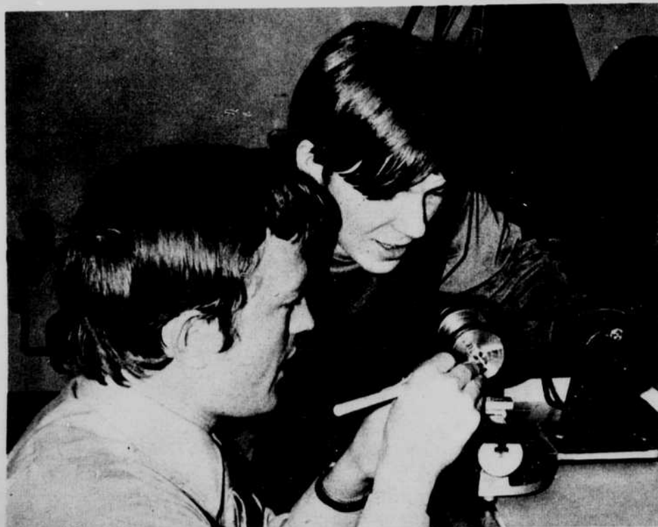
Assistant Instructor Bill McKeeth (foreground) is demonstrating the use of a "three-jaw precision chuck" to student Perry Good.
