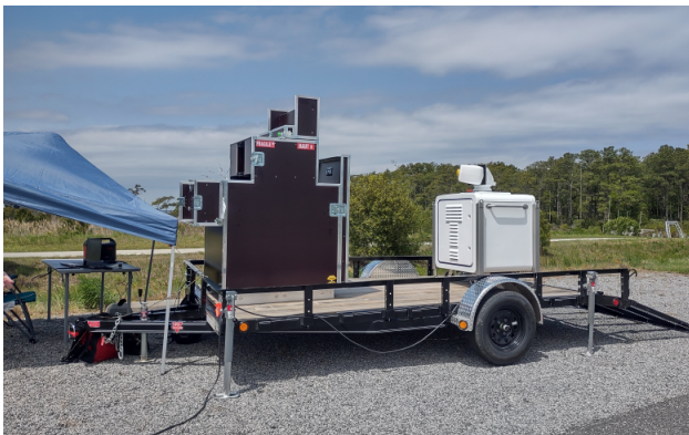
Figure 4: Windcube Scan 100s field-deployable scanning Doppler LIDAR
