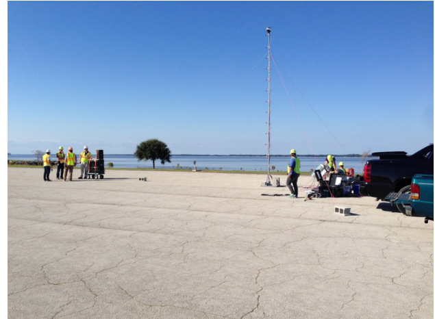
Figure 2: Portable mast with microphone array and associated weather station.
