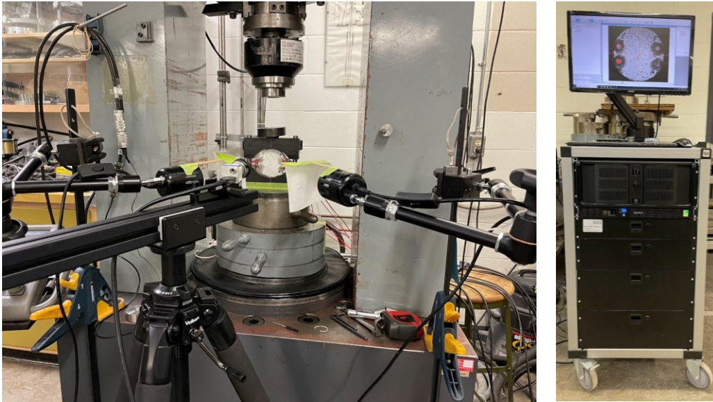
Fig. 2.6 Imaging system setup for the 2D DIC method
