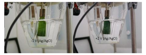
Fig. 9. Images of a sample of PES-Pani/HSO<sub>4</sub><sup>-</sup> conducting fabric: (a) in the reduced form at -1 V, (b) in the oxidized form at +2 V.
