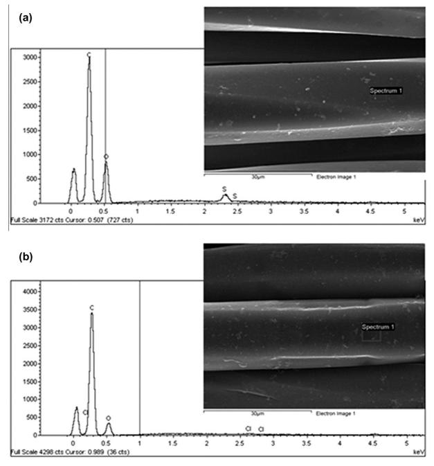
Fig. 4. Micrographs and EDX measurements of PES-Pani/HSO<sub>4</sub><sup>-</sup> (a) and PES-Pani/Cl<sup>-</sup> (b).
