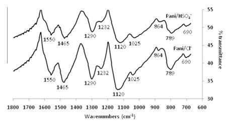
Fig. 1. FTIR-ATR spectra of Pani/HSO<sub>4</sub><sup>-</sup> and Pani/Cl<sup>-</sup> powders. Resolution 4 cm<sup>-1</sup>, 400 scans.
