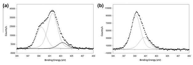
Fig. 5. XPS high resolution spectra for N1s for: (a) PES-Pani/HSO<sub>4</sub><sup>-</sup> and (b) PES-Pani/Cl<sup>-</sup>.
