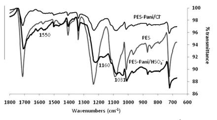
**Fig. 2.** FTIR-ATR spectra of PES, PES–Pani/HSO<sub>4</sub><sup>-</sup> and PES–Pani/Cl<sup>-</sup>. Resolution 4 cm<sup>-1</sup>, 400 scans.
