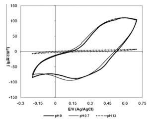
Fig. 8. Cyclic voltammograms of PES–Pani/HSO $_4^-$ , fifth scan for all measurements: 1 mV s<sup>-1</sup>; pH ~ 0, pH ~ 0.7, pH ~ 13.
