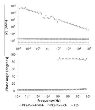
Fig. 6. Bode plots for PES, PES–Pani/HSO<sub>4</sub><sup>-</sup> and PES–Pani/Cl<sup>-</sup>. Sample located between two copper electrodes. Frequency range from  $10^5$  to  $10^{-2}$  Hz.
