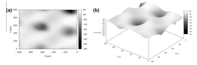
**Fig. 12.** 2D (a) and 3D (b) constant height SECM images of a PES–Pani/HSO<sub>4</sub><sup>-</sup>, 0.25 cm<sup>2</sup> geometrical area. These images were taken with a 100  $\mu$ m diameter Pt tip, in 0.01 M Ru(NH<sub>3</sub>)<sub>6</sub><sup>3+</sup> (pH 2.4) at a constant height of 60  $\mu$ m. The scan rate was 100  $\mu$ m s<sup>-1</sup> in comb mode; lengths of *x* and *y* lines were 1000 × 1000  $\mu$ m with increments of 50  $\mu$ m.
