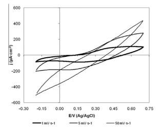
Fig. 7. Cyclic voltammograms of PES-Pani/HSO $_4^-$ , fifth scan for all measurements: 0.5 M H<sub>2</sub>SO<sub>4</sub> (pH  $\sim$  0); 50, 5 and 1 mV s<sup>-1</sup>.
