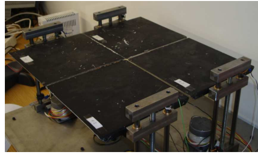
Fig. 4. Platform used to perform the various and different experiments. This platform is composed by four independent platforms, where it is possible to raise or drop each of them.
