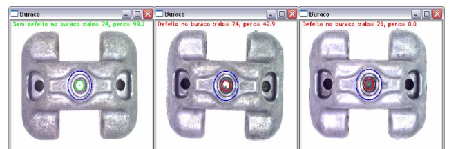
Fig. 13. Application of circular Hough transformation.
