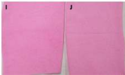
Figure 2: Cotton dyed with reactive dye (I) and with CNPs (J) at pH 8
