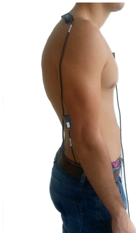
Figure 1. Inertial sensors' placement.
