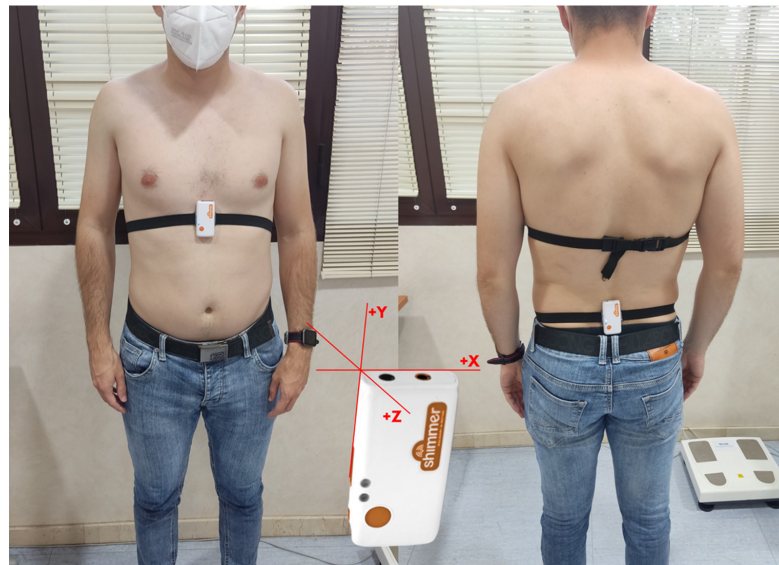
Figure 1. Shimmer 3 IMU: Placement and coordinate references (X, Y, Z axes).
