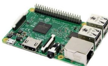
Figura 19. Raspberry Pi 3 Model B
