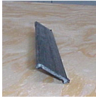
Fig. 9. U-Shape GF/PP pultruded profile made from towpregs
