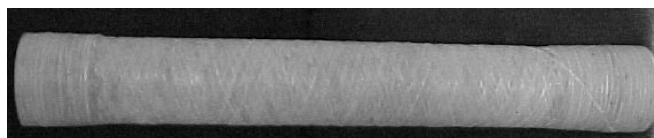
Fig. 8. Filament wound GF/PVC pipe
