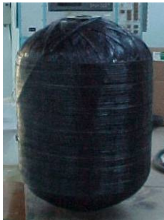
Fig. 7. Filament wound GF/PP pressure vessel processed from towpregs
