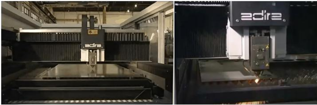
Fig. 3 – Framework runway beam of the laser machine during a cut.
