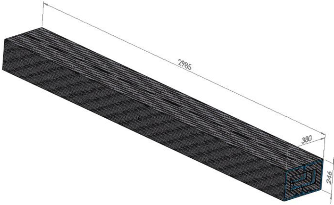
Fig. 7 – General view of the beam made of composite material (dimesnions in mm).
