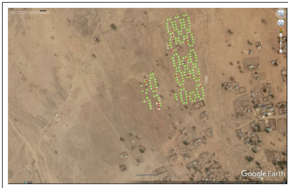
Figure 7. Detection of tents in a refugee camps, showing true positives (green); false positives and double detections (orange); and false negatives (red).
