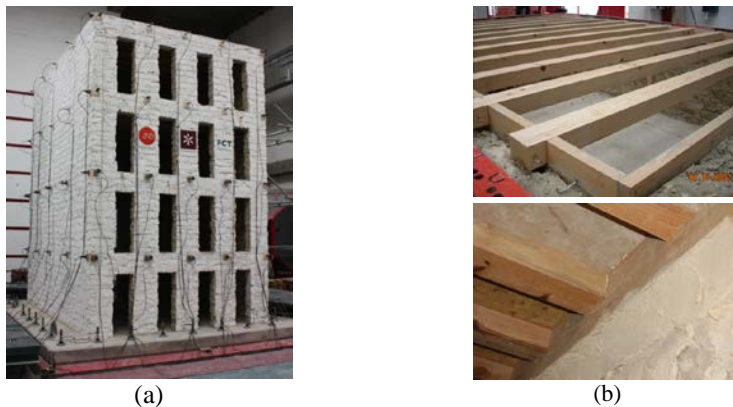
Figure 3: Mock-up building: (a) general view; (b) details of the floors.
