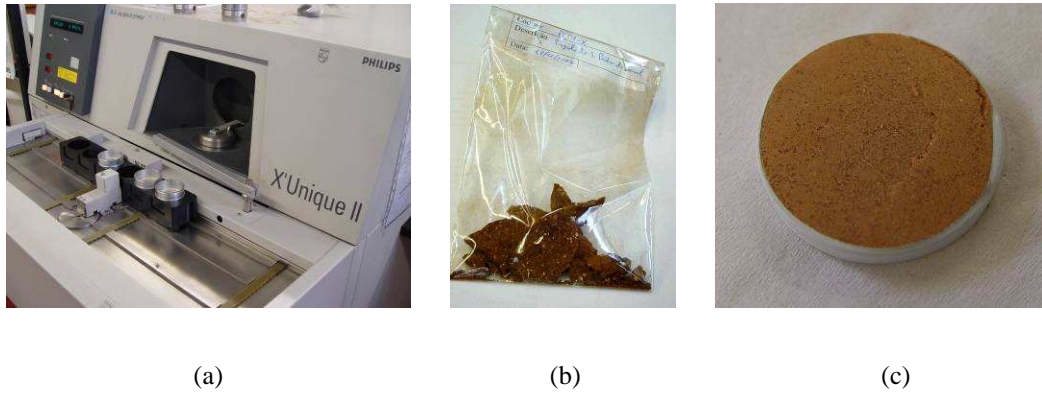
Figure 3 – Analysis equipment, X-Ray spectrometer, and preparation of the ceramic sample for spectrometry measurements. (b) Aspect of the sample extracted from bricks and (c) plastic tablet with the ceramic material ready for testing
