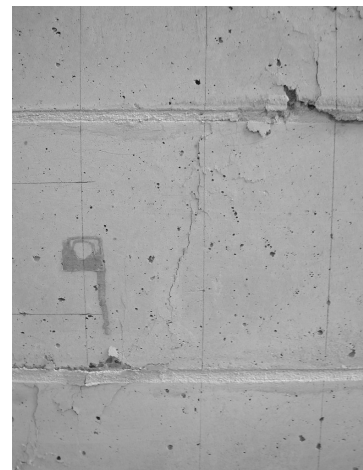
Fig. 4. Failure process: (a) Evolution of cracking in blocks and mortar crushing – dashed line indicates initial cracking, continuous line indicate the final cracking pattern and dark spots indicate mortar crushing; (b) details of cracking and crushing.
