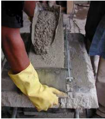
Fig. 3. Manufacturing of concrete beam and mortar sample.
