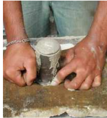
Fig. 3. Manufacturing of concrete beam and mortar sample.
