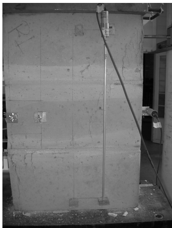
Fig. 4. Failure process: (a) Evolution of cracking in blocks and mortar crushing – dashed line indicates initial cracking, continuous line indicate the final cracking pattern and dark spots indicate mortar crushing; (b) details of cracking and crushing.
